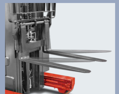
Forks can tilt forward/backward for easy loading
