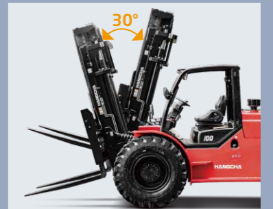
The tilt angle of the mast is 15° in the front/15° in the back, which is more suitable for loading, unloading and transportation of goods in off-road conditions
