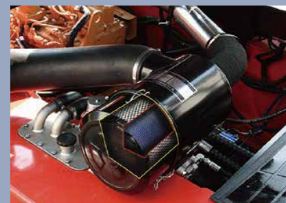
The novel high-flow air filter with a safety filter cartridge to enable cleaner air intake and higher power of the engine
