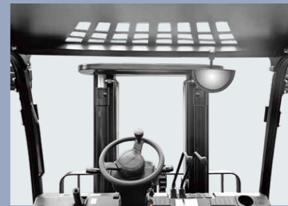
A wide-view mast system is used, the opening of the mast is widened, and the dashboard in the cab is lowered, so that the front view of the driver is broadened significantly
