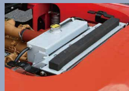
A plate-fin heat dissipater with high-performance fins is used to enable low oil and water temperature without water and oil leakage
